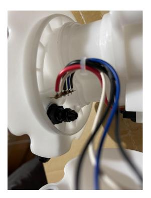
10. Now take your pressure regulator delete line and screw the -4AN female end to the bottom of the bulkhead fitting we just tightened down
