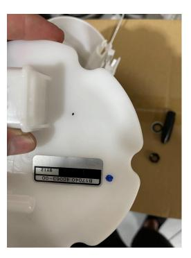
8. Being careful not to go too large and using a stepped drill bit, drill a 7/16 hole through the spot you just marked.
