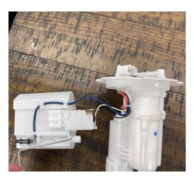
3. Remove the small white cap at the base of the pump, it is quite tricky. It is easiest to get a small plastic pry tool between the clip and the cap and gently pry away from the cap. Be careful, you still want the clips left intact as they will hold the new pressure regulator delete fitting in place.
