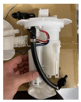
11. Make sure the o-rings are on the pressure regulator delete fitting and are well lubed. Take the delete fitting and install it into the port we took the fuel pressure regulator out of. There should be a satisfying click as the regulator clips into place.
