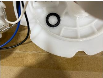
6. Besides grinding the webbing on the bottom of the hat we have to remove the majority of the three ribs on the side of the canister so our return line has room to squeeze in and not obstruct the basket from fitting and moving freely.
